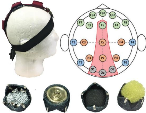
Figure 2.: BCI headset prototype (flexible headset, measured area, electrodes).
