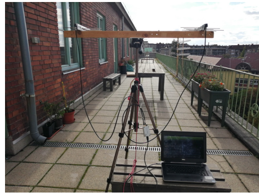
Fig. 15: The realized experimental model of the reflector's system.
