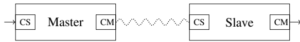
(a) Use-case for a wireless boundary clock, where the Slave device synchronizes to a Master device through UWB, and acts as a master device to other slaves.
