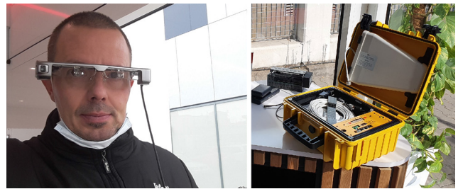
Fig. 5. AR Remote Trouble Shooting case with Epson's Moverio glasses
