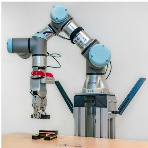
Fig. 1. Realized robotic system: An UR3e industrial robotic arm equipped with a RealSense D435i depth camera.
