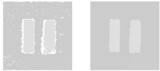
Fig. 3. Depth images of two jenga pieces as seen from above, before (left) and after (right) image processing.
