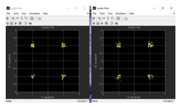
Fig. 21. Output scatter plots in Fig. 19. At the lower right corner of each scatter plot, it can be observed that these constellation diagrams were reconstructed at the very beginning of the simulation time
