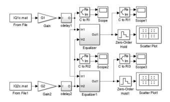
Fig. 19. The equalizer system diagram in Matlab. Input files containing data after synchronization, are IQ1c.mat and IQ2c.mat. Outputs are scatter plots of the equalized constellation diagrams
