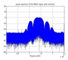
Fig. 13. FFT of the received signal without a pilot
