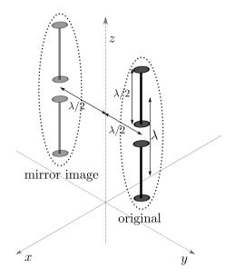
Figure 3. Constructing a simple directional antenna element from half-wavelength dipoles.
