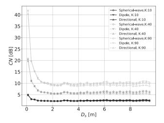
Figure 6. Condition number along with the element spacing of equidistant arrays for comparing propagation models.
