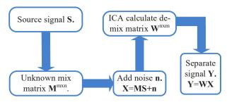
Fig. 5. Block diagram of ICA
