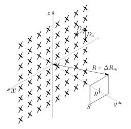
Figure 1. Scenario of 8 antenna element in the x-z plane,  $D_s = 1$  m. The EM field is evaluated on the S plane for different R.
