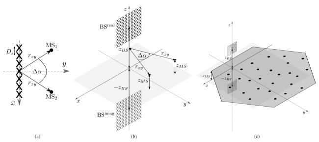
Figure 4. Different model scenarios. (a) depicts the one-dimensional case, whereas in (b), the two-dimensional case was drawn, with the mirror image antenna array utilized to model perfect reflection. In (c), uniformly distributed users are presented in a hexagonal cell.
