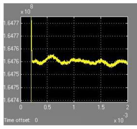
Fig. 10. The previous Figure, magnified. After settling, the frequency is kept within 1 kHz
