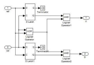
Fig. 7. The phase-frequency detector PFD in Fig. 6
