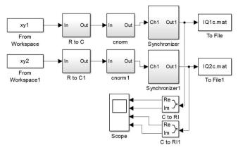
Fig. 17. The synchronization system in Matlab
