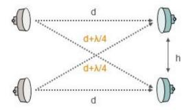
Fig. 1. The 2 x 2 MIMO concept. From d and the operation frequency, h is determined
