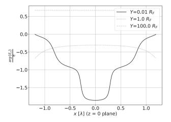
Figure 2. Illustrating the change in  $\arg\{E_z\}$ . In the near-field  $(Y = 0.01R_F)$ , there is an abrupt change in the phase and  $\arg\{E_z\} \in [-\pi, \pi]$ . In the transition zone  $(Y = R_F)$ , there is rather continuous change in the phase and  $\arg\{E_z\} \in [-0.918\pi, -0.307\pi]$ . In the far-field  $(Y = 100R_F)$ , the change in phase can be neglected compared to the change in the transition zone.
