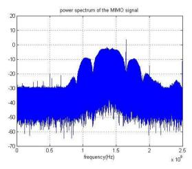
Fig. 3. FFT of the measured data with a pilot
