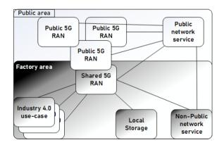
Fig. 2. Deployment with shared RAN and control plane
