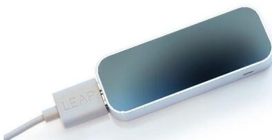
Fig. 2. The Leap Motion controller (source: [https://upload.wikimedia.org/wikipedia/commons/thumb/d/df/Leap\\_Motion\\_Orion\\_Controller\\_Plugged.jpg/440px-Leap\\_Motion\\_Orion\\_Controller\\_Plugged.jpg](https://upload.wikimedia.org/wikipedia/commons/thumb/d/df/Leap_Motion_Orion_Controller_Plugged.jpg/440px-Leap_Motion_Orion_Controller_Plugged.jpg))
