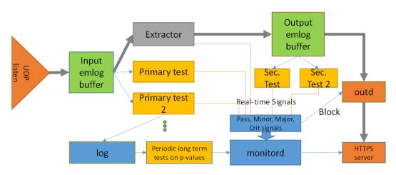
Fig. 2. Layout of the system and relations of the processes within. The thicker arrows show the path of the input data.
