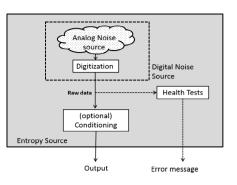
Fig. 1. General layout of a random number generator according to the NIST recommendation.
