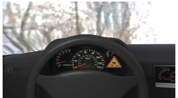
Figure 12. Visualizing situation-aware information in car instrumentation
