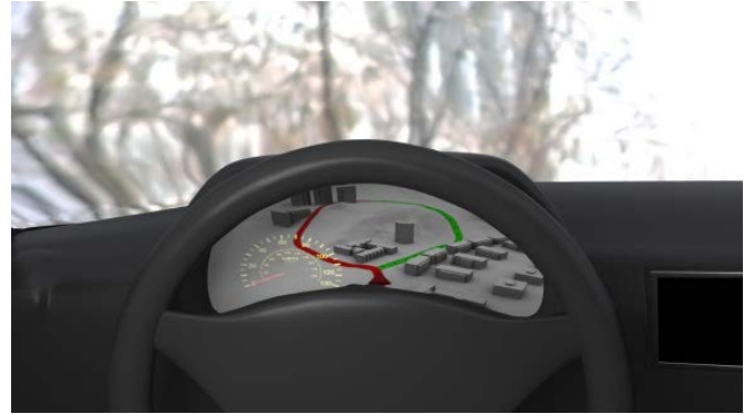
Figure 10. Visualizing route planning based on height curves (information needed in electrical cars with a low battery level)
