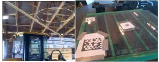
Figure 3. Transporter tracking with RFID tags in the ceiling or QR codes in the roof of a forklift truck
