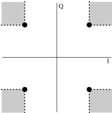
Fig. 2. ACE extension regions for QPSK modulation
