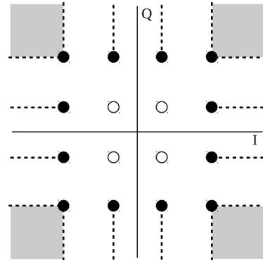
Fig. 3. ACE extension regions for 16QAM modulation
