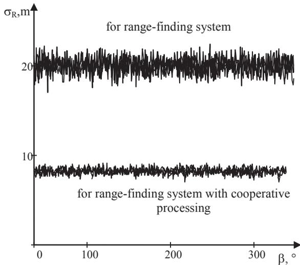
Figure 2 – MSE for range-finding of the object for different methods of measurements processing (for normal distribution)
