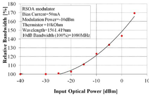
Fig. 4. Measured bandwidth improvement versus input optical power
