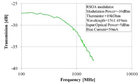
Fig. 2. Typical measured frequency response
