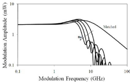
Fig. 9. Simulated modulation response for different mismatches
