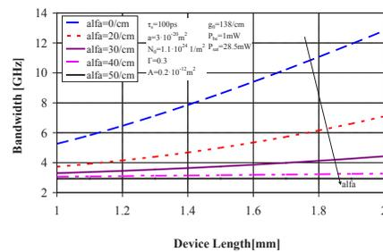
Fig. 7. Simulated bandwidth versus device length
