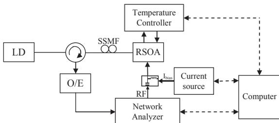
Fig. 1. Measurement setup
