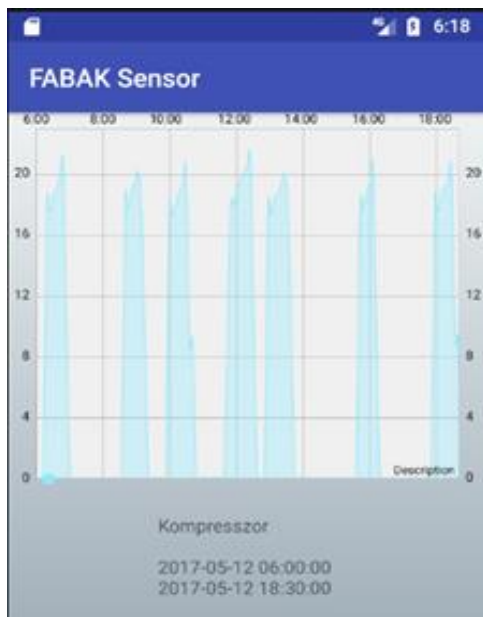
Fig. 6. Displaying IoT-related Amper data for a compressor in a Hungarian mobile application
