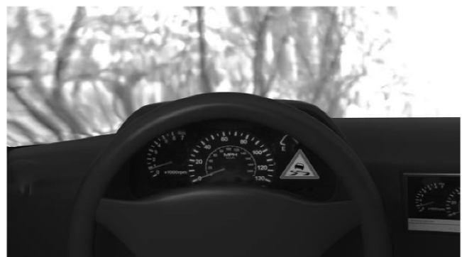
Figure 12. Visualizing situation-aware information in car instrumentation
