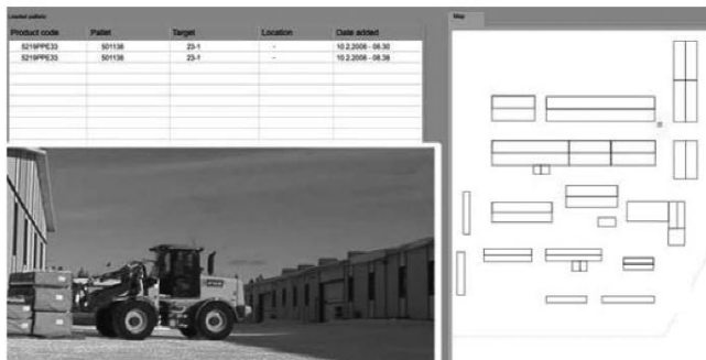
Figure 2. Smart wheel loader with location and product information and RFID tags inside warehouse
