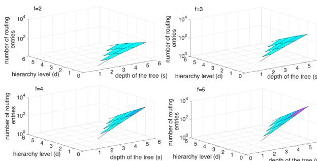
Fig. 3: Scaling of routing entries in a specific node in the RPL DODAG as the function of its hierarchy level  $d$  and the depth of the tree  $s$ , in case of an increasing number of children  $f$  and a full tree
