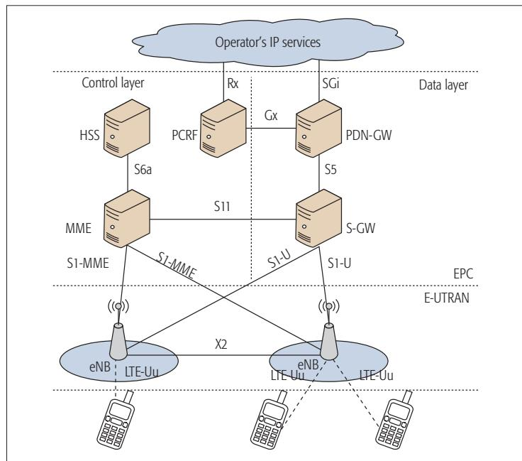
Figure 1. The (basic) 3GPP evolved packet system.
