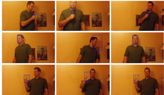
Fig. 2. Experimental realization of tracking the head, microphone and hand based on CMT algorithm.
